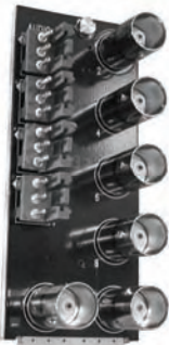
Figure 4. AES-BNC Rear I/O Module
