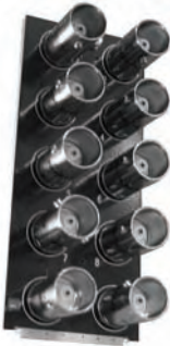
Figure 5. 10 BNC Rear I/O Module
