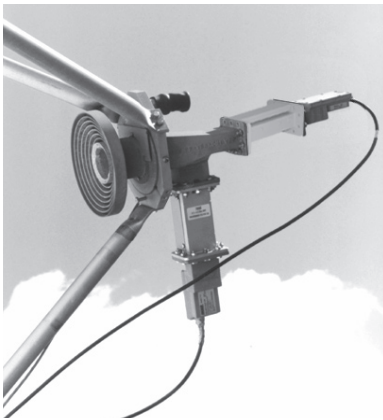
Photo of 8523D (8524D) mounted between antenna feed and LNA's (both Vertical and Horizontal Polarization.)
